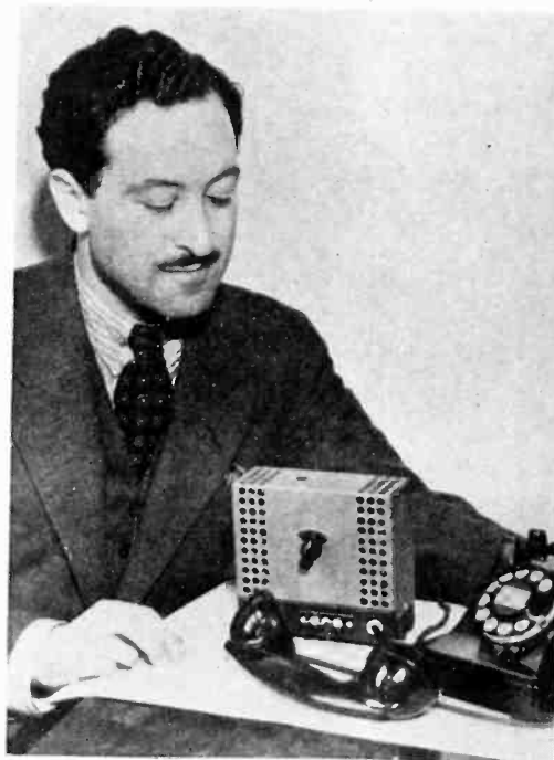
Archie Baxter using the interphone set in his trailer flying school outdoor "operations headquarters" at Floyd Bennett Field. The interphone connects the trailer with a small office he has in the airport Administration Building about a mile and a half distant. In this manner Baxter keeps in touch with what is going on at the airport
