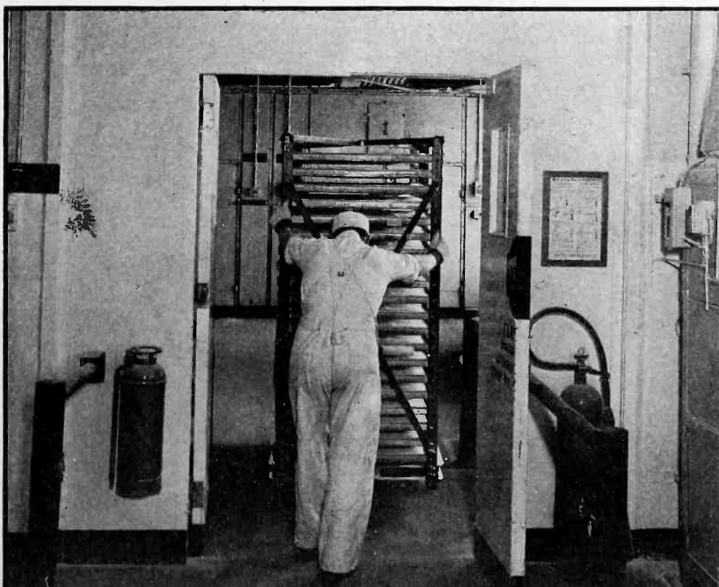
As the worker approaches this door he steps into a light beam. The door then opens and remains open until both the worker and the truck have completely passed through the door
