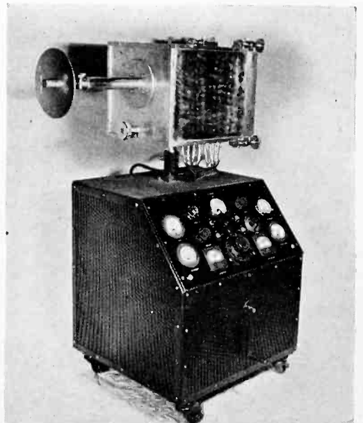
Generator for operation in the 3000 to 4000 megacycle region at the R.C.A. plant at Camden and used by research engineers for studying centimeter wave detection measurements and performance
