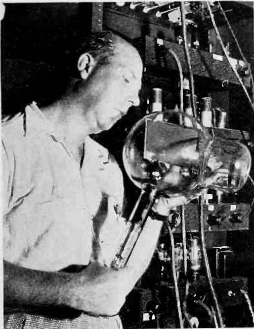
Prof. W. L. Everitt, Ohio State University radio authority, studying the construction of an iconoscope at the Armour Institute of Technology at Chicago where defense classes are being held
