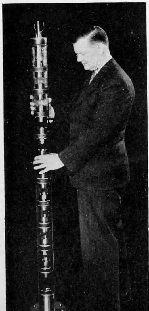
Fig. 8—A million-volt x-ray tube. Multi-section construction is used to distribute the voltage gradient uniformly
